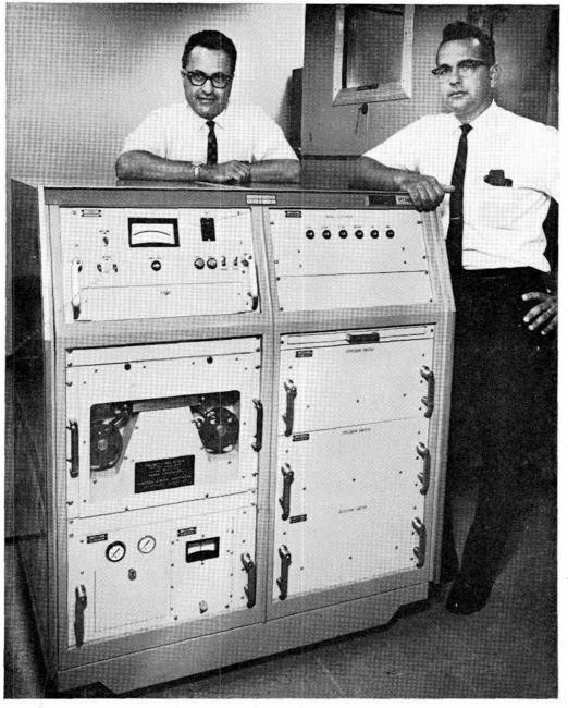
NEW TESTER — Prototype of a new breed of production tester based on fluidics technology is displayed by Gino Carli (left), Division 2451 supervisor, and Ron Oelsner, tester designer.
